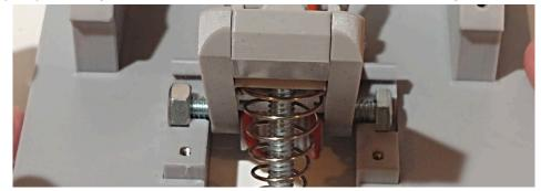
**Step 10** - Hook the axle drive band around one of the axle bracket forks to keep it out of the way, then put the sanding spindle back through the other band, the one that is only around the idler pulley, so that the band is now on the center pulley of the sanding spindle. Make sure the large pulley is on the motor end, like it was before.
