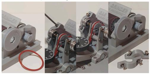
**Step 8** - Press down on the center of the paddle in front of the indicator knob, compressing the spring. This will help you lift the sanding spindle out of its supports so that you have access to the tramming screws, one in the center of each support, below where the roller bearings rest. You should be able to release the axle bracket with the sanding spindle pinned between it and the spindle supports.
