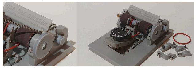
**Step 5** - Unscrew the indicator knob completely, removing it, so that both the axle bracket assembly and sanding spindle can be removed from the base. If the sanding spindle band is still in one piece, the spindle can now be easily removed from it.
