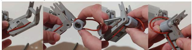
**Step 9** - Test fit the axle bracket into the clamps. You will probably need to adjust the nut in or out a little bit for a good fit. It should be snug and not loose, but a little loose is OK. Don't clamp it in just yet, though! Take it back out of the base to refit the sanding spindle.
