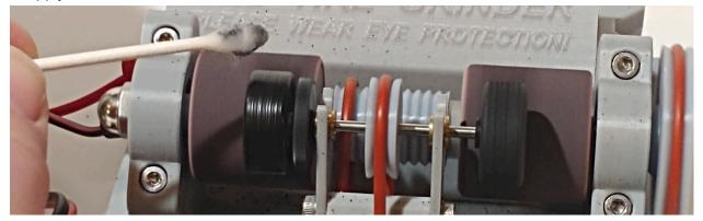
**Step 10** - Without changing the position of the indicator knob, repeat step 9 as often as necessary until there is very little difference between the pitch and amp draw when the tire is wet with IPA and when the tire is dry. At that point, turn off the machine and check the tires for progress. Note the current position of the indicator knob, which might come in handy later.
