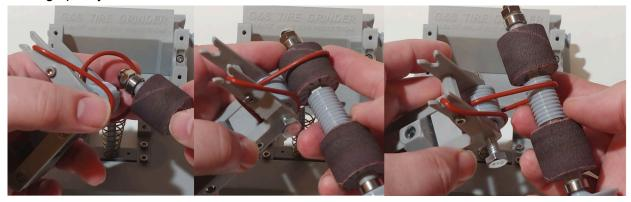
**Step 11** - Put the sanding spindle back into the supports, and the axle bracket onto the adjustment bolt. Don't worry about the axle bracket pivot bolt yet. It can be up in the air for now.
