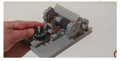
**Step 2** - Using your 2.5mm hex driver, remove the screw from the axle bracket pivot clamp on both sides of the axle bracket assembly. Set the screws and clamps aside.
