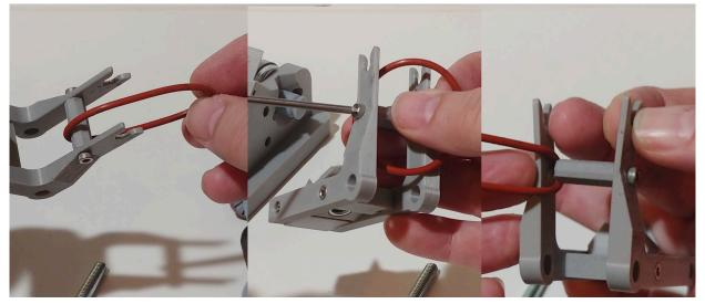
**Step 8** - Move the axle drive band out of the way by looping it around the paddle end of the axle bracket. Reinstall the idler pulley with the other replacement band around it, holding it in place while reinstalling the pivot bolt and nut. Leave the nut near the end of the bolt.
