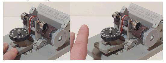
**Step 9** - Using your 2.5mm hex driver, unscrew (back out) the tramming screw (m3x6mm socket head cap screw) on the side that the paper was able to slide freely. The goal is to raise that bearing just enough for that side to have the same amount of friction on the paper as the other side. Since the screws are normally not touching the bearing at all, start by unscrewing it by 1.5 full counterclockwise rotations. Use a reference point on your driver to confirm how much you are turning it.
