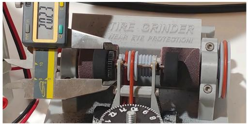
If the difference in diameter is negligible, e.g. under 0.1mm difference, but with one tire needing more work, or your goal is to get the tire to a specific outside diameter for competition, then continue with repeating steps 10 and 11 while adjusting the indicator knob a little bit at a time until both tires are evenly sanded all the way across and all the way around and are both of the same target diameter.
