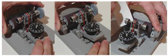
**Finish** - Replace the sanding spindle clamps and the four screws. It is best to start all four screws, making sure not to cross-thread any of them, screwing them in evenly until you feel resistance. Do not screw them down hard, especially on the side that required adjustment. Doing so may distort the bearing and cause problems using the machine, and excess wear on the bearing. Check the tramming one more time with the paper before proceeding.
