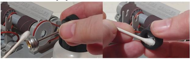
**Step 4** - Glue the tires to the wheels. This can be tricky, so it can help to have glue that does not bond too quickly like common super-glue (cyanoacrylate) tends to. A popular product that many slot racers prefer is Gorilla brand super glue, easily identified by the blue colored cap on the bottle. It is thick and does not cure instantly, providing good working time for the process.
