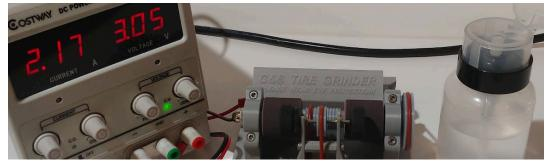
The pitch will go down, while the amperage will go up, as soon as the tires contact the sanding drums. Do NOT apply excessive pressure to the sanding drums with the tires. Doing so will cause the machine to stall, or the axle to skip or stutter, which can damage the tires or the machine. Slow and steady is best.
