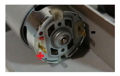
When connecting the output of the power supply to the G&S Tire Grinder motor, the positive lead should be connected to the left terminal of the motor (when viewed as shown in the photo), and the negative/ground should be connected to the right terminal. The terminals are 3mm, and can be soldered to, clipped to with alligator clips, or connected using 3mm, 5/32", or 3/16" female spade connectors.
