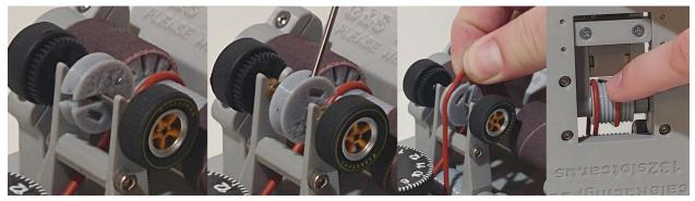
Before continuing, it's best to lubricate the bushings or bearings. Use your favorite light oil, such as 3-in-1, INOX MX3, or any number of similar products, whether they're marketed to slot car racers, or RC racers, or whatever. A single drop for each bushing should be plenty. You can manually turn the axle, or turn on the machine at a low speed/voltage to help the lubricant wick into the space between the axle and bushing.
