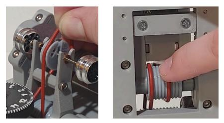
**Step 4** - Turn the indicator knob counterclockwise so that the wheels move closer to the sanding spindle drums. Keep turning until one wheel is just touching the sanding drum, then turn the knob clockwise a small amount so that there is a thin space between the wheels/tires and the sanding drums.
