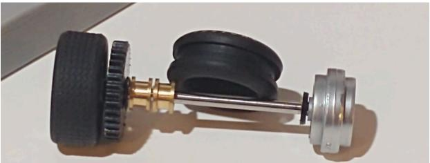
**Step 2** - Tires can also have imperfections from the molding process, not only on the outside, but also on the inside. Examine the tire thoroughly and clip off any obvious bits of flashing or imperfections. In some cases, it's helpful to turn the tire completely inside out to clean those surfaces.
