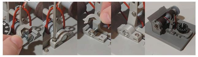
**Step 15** - Last, but certainly not least, replace the main drive band by first wrapping it around the large pulley on the end of the sanding spindle, and then stretching it out and over the small pulley on the drive motor.
