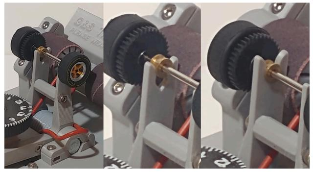
**Step 6** - Install the appropriate split pulley (3/32" and 3mm options are provided with pre-installed nuts and set screws) as close to the center of the axle as possible. If there is a gear in the center of the axle already, just put the split pulley to whichever side seems to work best. Use a 1.5mm hex driver to tighten the set screw to the axle, securing the pulley.
