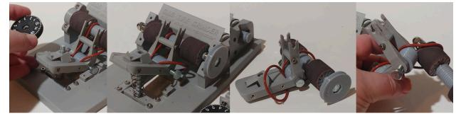
**Step 6** - Remove the nut from the end of the axle bracket pivot bolt, then remove the bolt so that the idler pulley can come out from between the axle bracket sides. If you only need to replace the band between the idler pulley and sanding spindle, you can skip to step **8**.
