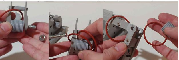
**Step 7** - If you need to replace the axle drive band, then you have another screw to remove. Use your 2.5mm hex driver to remove one of the screws from one side of the axle bracket, up near the forks, to release the stabilizing bar on one side. You can then gently pry that side of the axle bracket away from the stabilizing bar enough to slip the band between them, replace the band the same way, then replace the screw.
