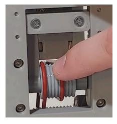
**Step 4** - Turn the indicator knob counterclockwise so that the wheels move closer to the sanding spindle drums. Keep turning until one wheel is just touching the sanding drum, then turn the knob clockwise a small amount so that there is a thin space between the wheels/tires and the sanding drums.
