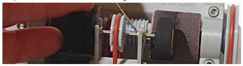
**Step 7** - Make sure the tires are NOT touching the sanding drums, and then turn on your power supply unit (PSU), setting the voltage to approximately 3V, no more than 4V. If your PSU has an amperage display, take note of the value while the machine is running without the tires touching the sanding drums. Otherwise, pay attention to the pitch of the motor as it's spinning.
