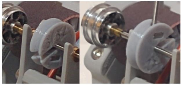
**Step 3** - Pull the rubber band over the wheel and bracket and onto the split pulley. Through the opening on the base of the machine, you can roll the band to either side so that the wheels are centered on the axle bracket.
