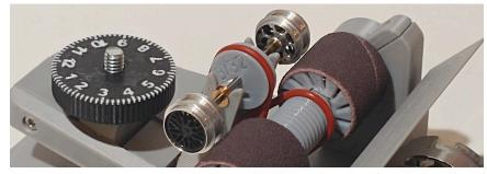
**Step 5** - Using a piece of paper, such as regular printer paper or a post-it note, slide the paper between the wheel and the sanding drum on both sides. If the paper slips freely between them on both sides, turn the knob back slightly until the paper can still move, but you can feel friction. The paper should not be trapped by the wheel and sanding drum, but there should be a slight resistance to pulling it, while still being able to push the paper through the gap.
