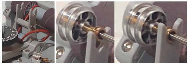
**Step 2** - Install the appropriate split pulley as near to the center of the axle as possible. A set screw is provided, or already installed, requiring a 1.5mm hex driver to adjust. Snug down the set screw.
