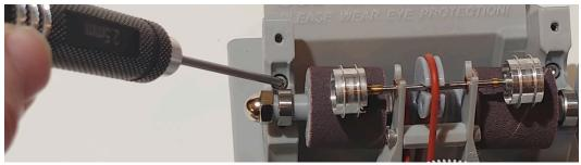
**Step 10** - Press and release pressure on the axle bracket while replacing the sanding spindle and hold it firmly in place on the supports while testing both sides with the piece of paper again. You should only need to test the side you are adjusting, but it is also a good idea to test both sides before determining that tramming is complete. Repeat steps 8-10 with small adjustments to the tramming screw until both sides have the same amount of friction for the paper.
