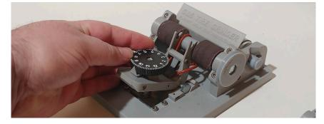
**Step 4** - Remove both screws from the clamps at both ends of the sanding spindle. Set the screws and clamps aside.
