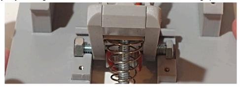
**Step 10** - Hook the axle drive band around one of the axle bracket forks to keep it out of the way, then put the sanding spindle back through the other band, the one that is only around the idler pulley, so that the band is now on the center pulley of the sanding spindle. Make sure the large pulley is on the motor end, like it was before.
