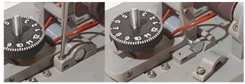
**Step 3** - Turn the indicator knob counterclockwise to raise it up, allowing the axle bracket pivot bolt to lift up out of the clamps so that the entire axle bracket moves toward the sanding spindle until the rubber band between the two (if it hasn't broken) is loose.
