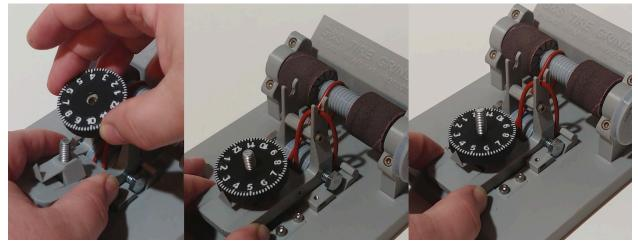
**Step 14** - Replace the clamps on the ends of the pivot bolt. Note that they are mirrored, and will only go on the correct side.
