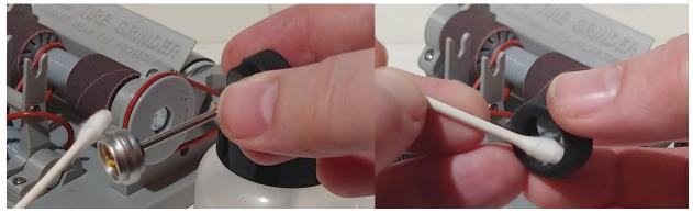
**Step 4** - Glue the tires to the wheels. This can be tricky, so it can help to have glue that does not bond too quickly like common super-glue (cyanoacrylate) tends to. A popular product that many slot racers prefer is Gorilla brand super glue, easily identified by the blue colored cap on the bottle. It is thick and does not cure instantly, providing good working time for the process.
