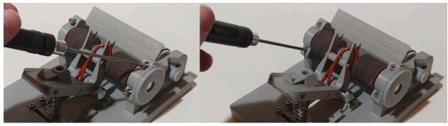
**Step 13** - Replace the indicator knob and turn it down to force the axle bracket into place. As you are doing so, make sure the pivot bolt is lining up with the clamps below, adjusting the nut at the end as needed. Again, it should be snug, but not hard to press into place. A little loose is ok, because the clamps will keep the nut and bolt from turning apart. Tighten the indicator knob as much as you need to so that the pivot bolt is firmly in place.
