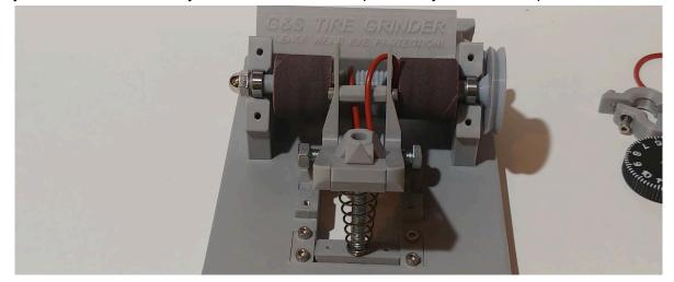
**Step 12** - Replace the clamps at both ends of the sanding spindle, being careful not to cross-thread the screws. Tighten them down evenly until you feel resistance to tightening. They should not need to be tightened down hard, as doing so may deform the bearings and cause problems or excess wear.
