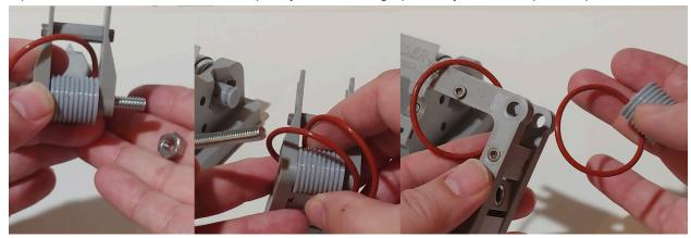
**Step 7** - If you need to replace the axle drive band, then you have another screw to remove. Use your 2.5mm hex driver to remove one of the screws from one side of the axle bracket, up near the forks, to release the stabilizing bar on one side. You can then gently pry that side of the axle bracket away from the stabilizing bar enough to slip the band between them, replace the band the same way, then replace the screw.
