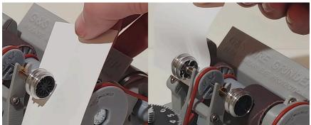
Now, test the other side. If either side is harder, or easier, to slide the paper between the wheel and sanding drum, then the sanding spindle is not parallel to the axle bracket, and one side will need to be adjusted. If both sides have the same feeling of resistance to moving the paper in and out, then the sanding spindle is already trammed, and you can skip to truing your first set of tires!
