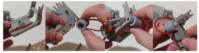
**Step 9** - Test fit the axle bracket into the clamps. You will probably need to adjust the nut in or out a little bit for a good fit. It should be snug and not loose, but a little loose is OK. Don't clamp it in just yet, though! Take it back out of the base to refit the sanding spindle.
